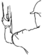
Screw stud to top and bottom track with screws, holding flange to track for easier attachment.
